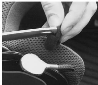
Carefully cut a small hole in the outer edge of the foam windsock so you can slide the microphone red connector and then boom through it, taking care not to tear it. Carefully position the foam over the fabric microphone covers so that the beige cover part is exposed.
